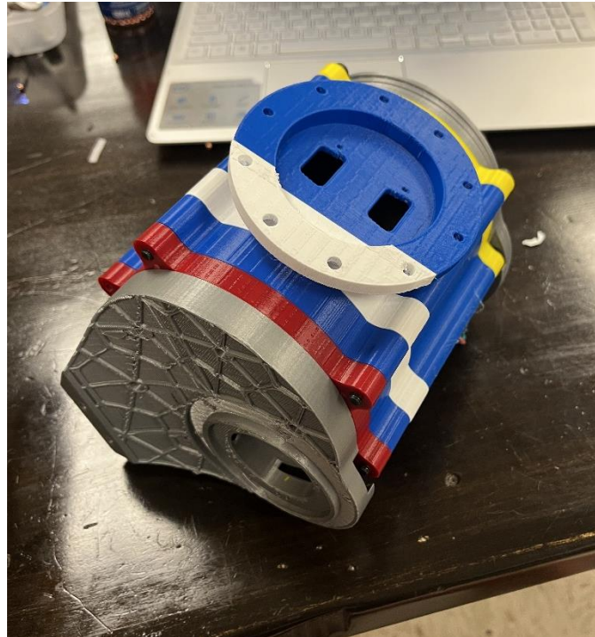
Fig 42. Completed shoulder joint assembly
